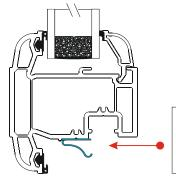
Fit a **BC001** Sash Spring to the sash on the center line of the stay fixing
