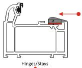
Fit a Frame Wedge "A" to include the packer "C" on the outer frame in the stay fixing area as shown
